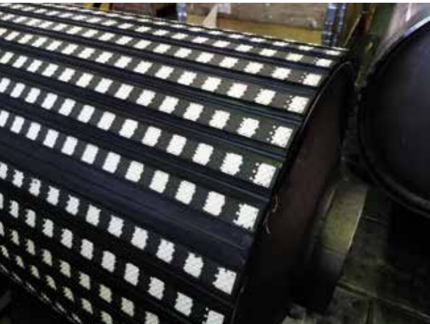
CK-X (ceramic tiles inside rubber)
