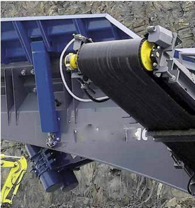
Rulmeca Motorized Pulleys in mobile Crushing & Screening. Features: Compact, reliable and requires NO maintenance!
