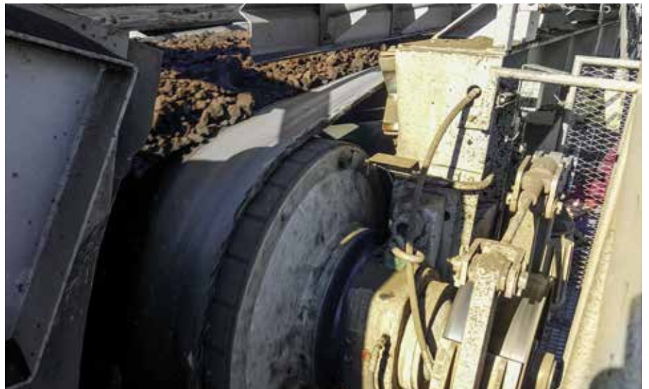
Excavators in different applications are using Motorized pulleys with driving power up to 250 KW. Compact design and equal weight distribution gives the design engineer a lot of options to create an efficient solution.
